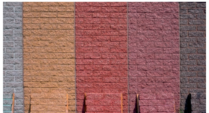
Concrete bricks (unweathered comparison sample in the foreground). Start of weathering exposure: 1970, photo: 1995.
