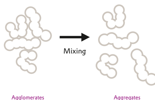
FIGURE 6: Agglomerate structure of AEROSIL® Pharma products
