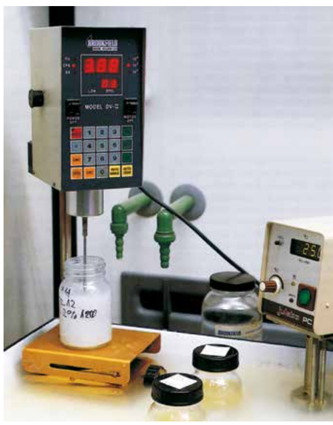
Figure 9 Rotation viscometer DV-II of the Brookfield Engineering Laboratories, Inc., 240 Cushing St., Stoughton, MA 02072 USA
