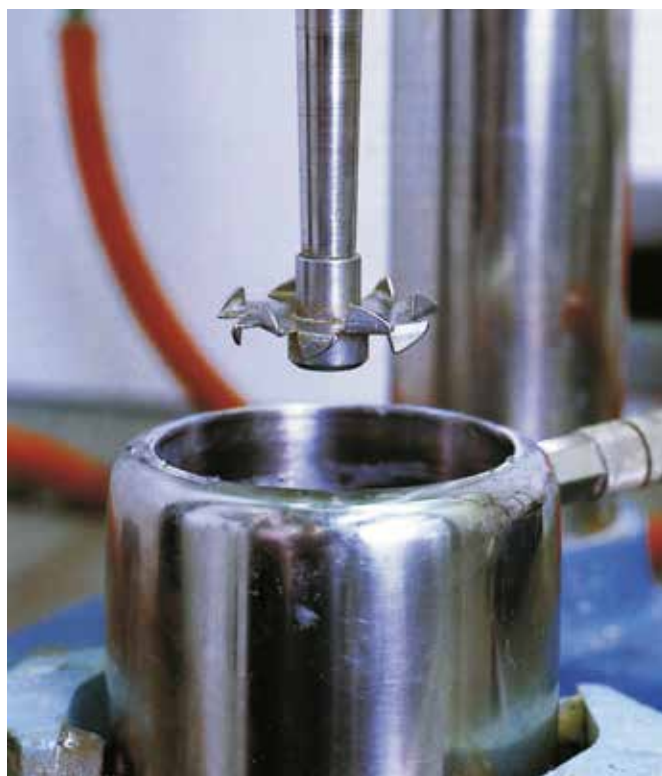
Figure 10 Lab dissolver blade (Cowles-Dissolver, Co., Morehouse, N. Y.)
