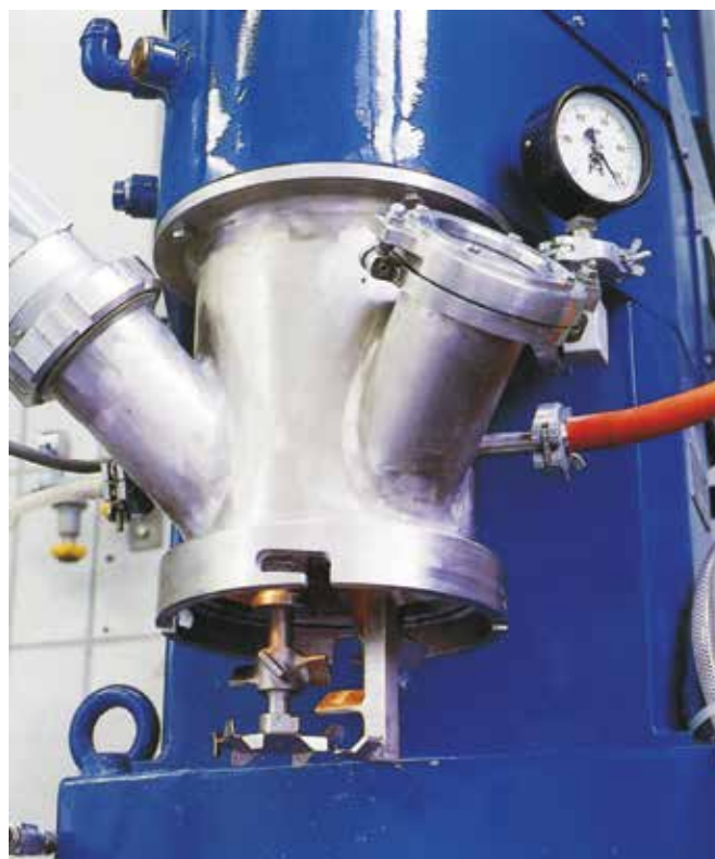
Figure 11 Lab planetary dissolver with vacuum- and inert gas equipment (Hermann Linden GmbH & Co., KG, 51709, Marienheide, Germany)
